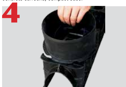
4 Push-fit outlet adaptor into bottom of channel, lay outlet channel first and connect to 4" or 6" SDR or schedule 40 pipe (Adaptor required for Sch 40).
